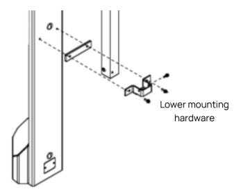
7. Screw the 1/4"Ø hex-head self-piercing screw on the side of the cable management column.
