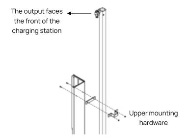
**RECOMMENDATION**: To position the column, make sure the cable management cable clamp is facing the front of the charging station/pedestal.
