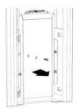
5. Remove the nuts (4), washers (4) and bolts (4) from the backside identified in step 3. Install the rectangular spacing shim on the pedestal upper mounting holes. Put the column in place then install the column mount bracket on the column. Screw the parts together loosely with the Phillips flat-head 1/4-20 screws and nylon locknuts. The CMS column is maintained in place and can move freely to install the lower mounting hardware.
