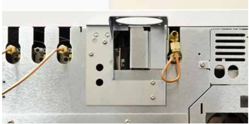
Figure 13 Bracket 5003-1356 installed to 7890 GC
