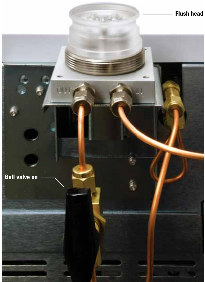
Figure 27 Using the flush head to flush the gas line of oxygen and moisture
