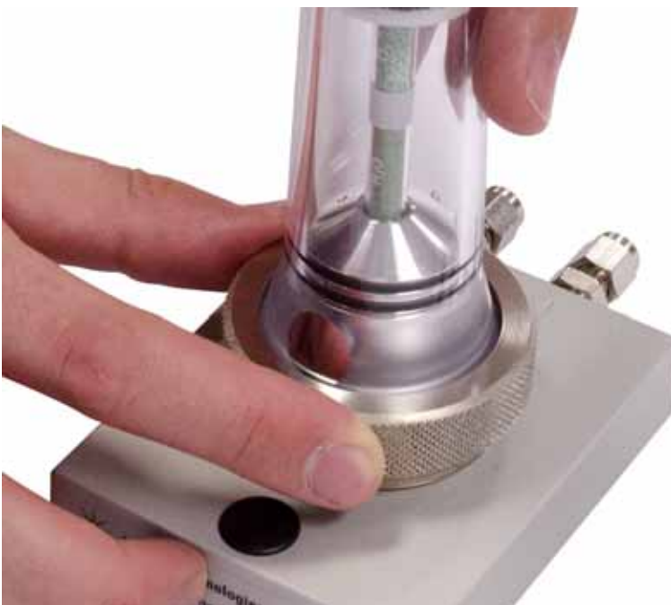
Figure 37 Unscrew the knurled or plastic ring nut
