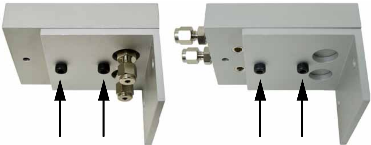
Figure 10 Hex screws installed
