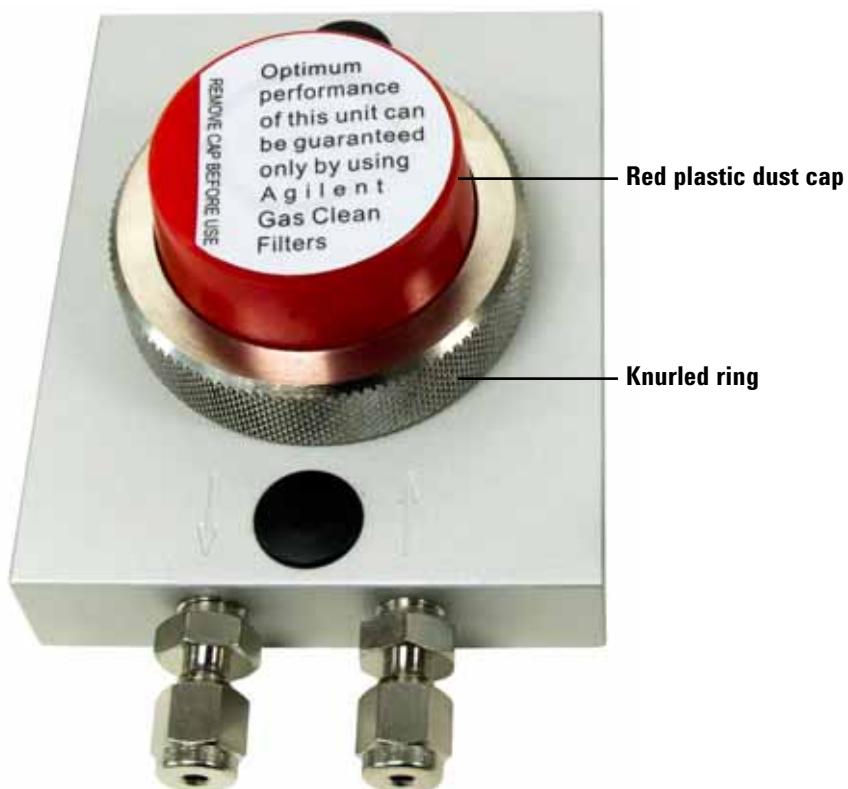
Figure 20 Remove the red plastic dust cap
