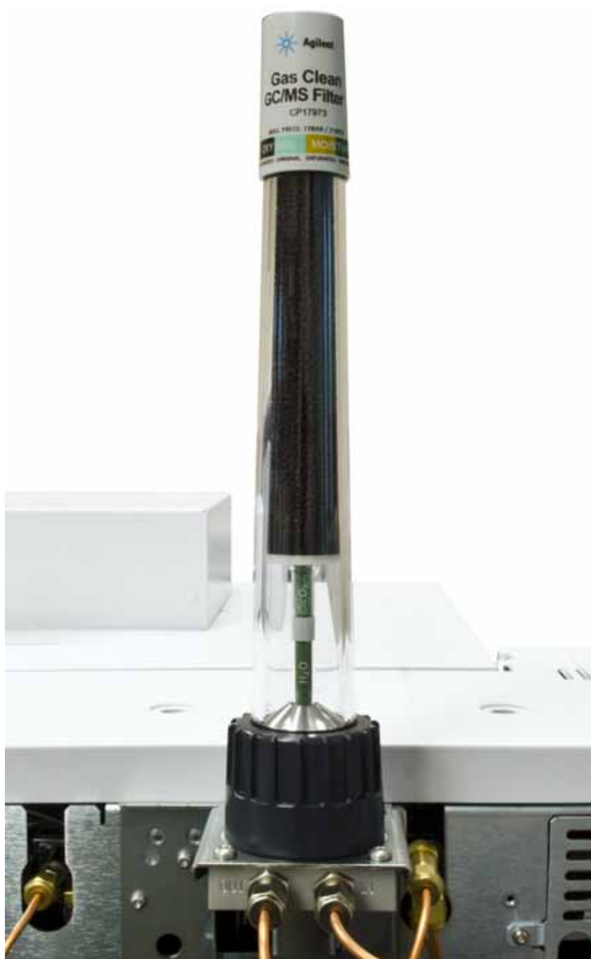
Figure 31 GC/MS filter installed to the bracket connecting unit
