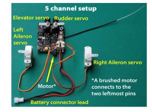
two tail control surfaces. Rudder input causes the servos to rotate in the same direction for yaw, while elevator input moves the two servos in opposite directions for pitch.<sup>3</sup> See Mixer Settings for details.
