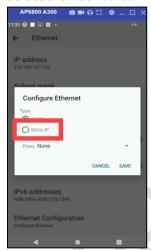
3. To manually set the IP address, select **Static IP**, enter the network information, and select **SAVE**:
