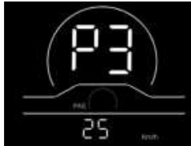
Fig. 4-3 Speed Limit Setting Interface
