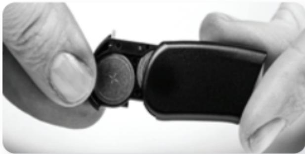
Then begin to attach the battery cartridge to the Naída CI by holding the sound processor in one hand. Rotate RF cable upward to avoid bumping it upon battery placement.
