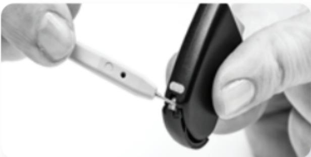
Set the tool aside. From here you can grasp the Zn-Air drawer with your hand and gently pull it the rest of the way out, so you are able to insert the Zn-Air cells.
