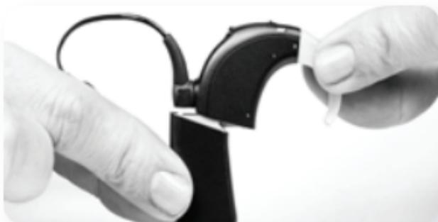
Align the battery cartridge connector with the processor housing side of the connector.
