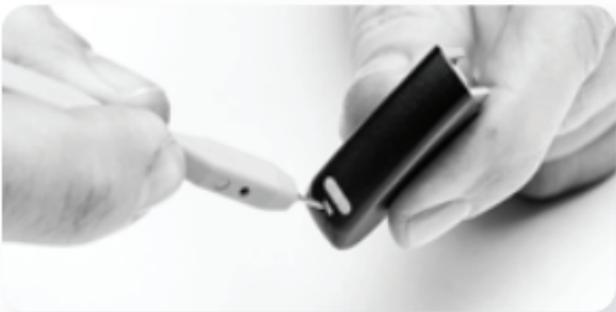
With the tool inserted in the hole, gently push in and downward until you feel the Zn-Air drawer release and pop out the button of the Zn-Air cartridge. If you do not have the tool present, any thin, pointed device should work to release the drawer.
