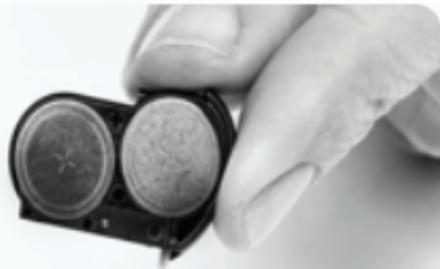
Once batteries are flush with the top of the battery drawer, gently slide the battery drawer back into the battery cartridge. If the cells are inserted incorrectly, the battery drawer will not close.
