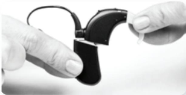
Align the battery cartridge connector with the processor housing side of the connector.
