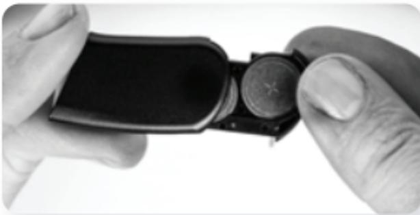
Then begin to attach the battery cartridge to the Naída CI by holding the sound processor in one hand. Rotate RF cable upward to avoid bumping it upon battery placement.
