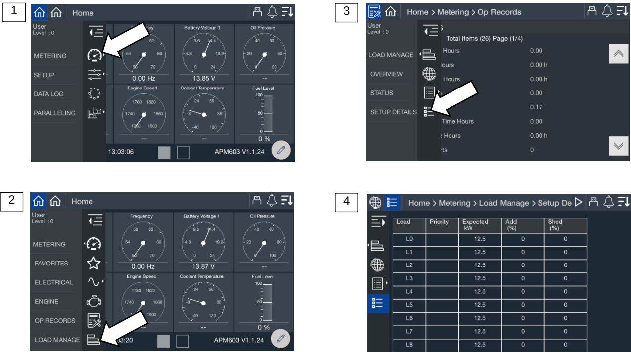
Figure 39 Metering, Load Management, Setup Details
