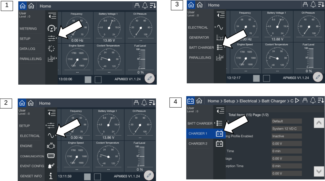
Figure 43 Battery Charger Setup Screen
