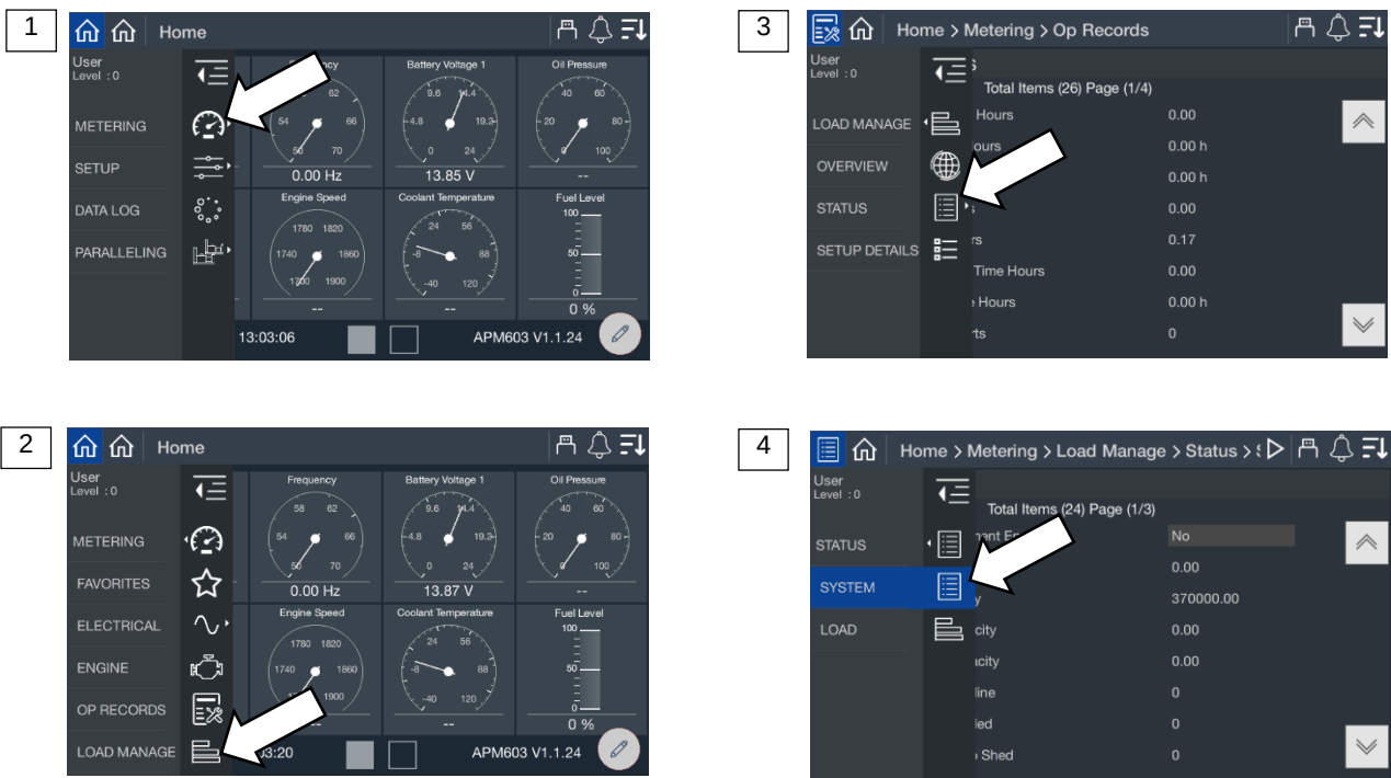
Figure 35 Metering, Load Management, Status, System
