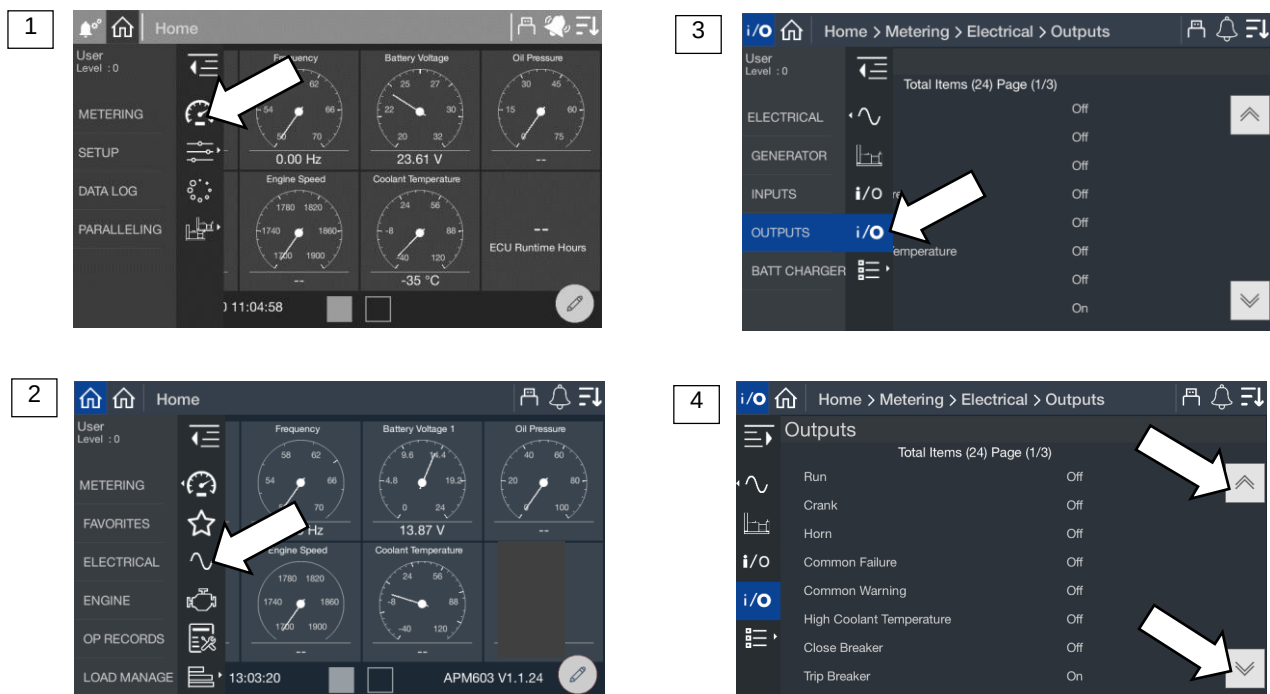
Figure 26 Outputs Metering Screen
