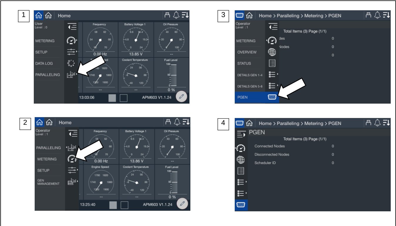
Figure 61 Paralleling, Metering, PGEN
