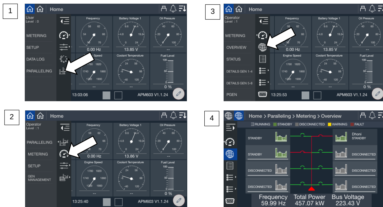
Figure 56 Paralleling, Metering, Overview Screen
