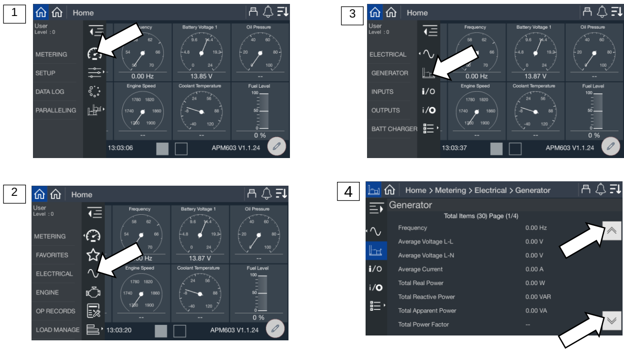
Figure 22 Electrical Metering Screen
