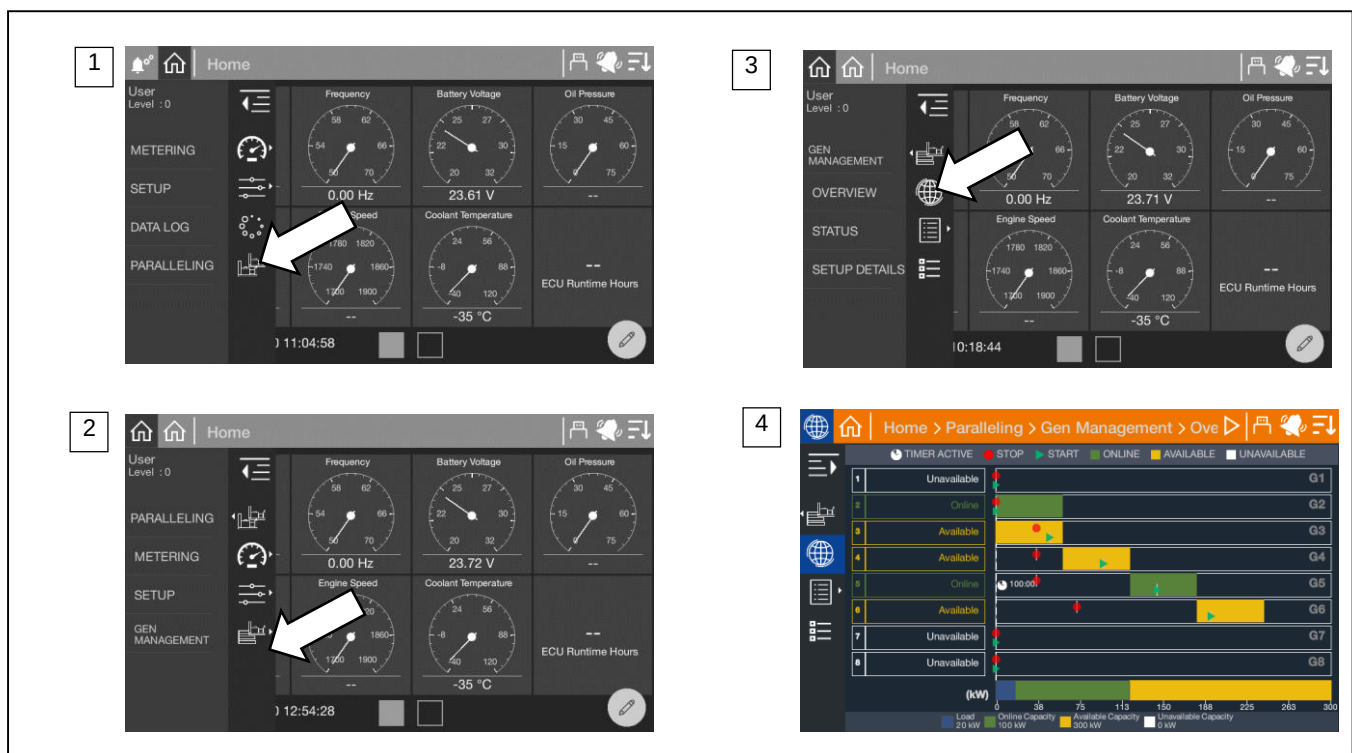
Figure 67 Paralleling Screens, Gen Management Overview
