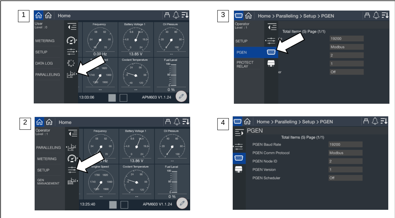
Figure 63 Paralleling, Setup, PGEN Screens
