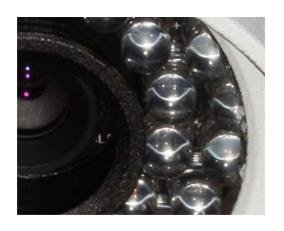
30 Infrared LEDs
