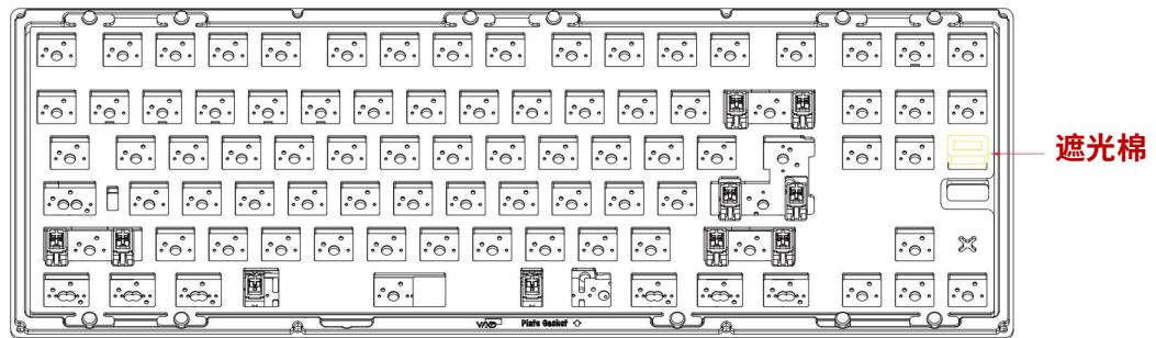
**6. Install switches, inter structure has been build. Put 2mm poron and 2mm hotswap poron into bottom case, connect the PCB with TYPE C.**
