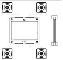
roc4ML-Pro can also work as a multiple SPI camera adapter. Up to 4 Arducam sga SPI cameras can be connected to the Pico4ML-Pro simultaneously.
