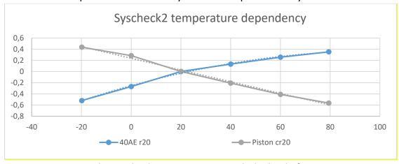
40AE r20: is the Syscheck2 measurement with the load of 40AE Piston cr20: is the measurement of the 40AE sourced by the pistonphone.
