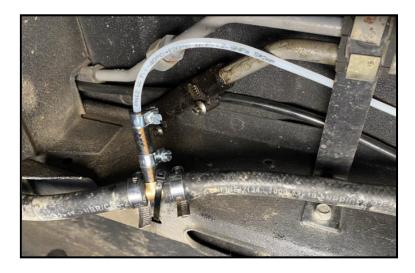
18) Grab the intake hose, filter, (2) hose clamps and assemble as pictured below.
