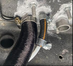
20) Route and secure the rest of the assembly under the vehicle using the Adel clamps or zip ties.
