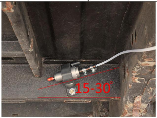
Attach the rubber fuel line to both ends of the fuel pump with the provided clamps.
