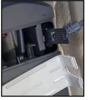
37) Position the grommet with the round side facing up. Slip the first groove into the heater, slip the grey cover on top, and make sure the cover slips onto the grooves.
