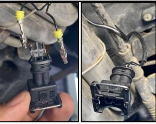
25) Connect one end of the fuel pump harness to the connector you just assembled and the other end to the fuel pump. Use zip ties to secure any excess harness neatly.
