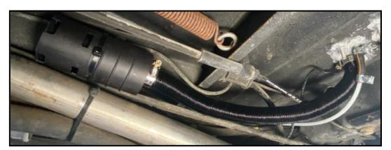
21) Next, get the steel exhaust hose and exhaust clamp, and secure one end to the heater's aluminum body port.
