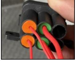
31) Connect the main power to the positive power supply on your auxiliary battery. Ground the brown wire anywhere on the vehicle.
