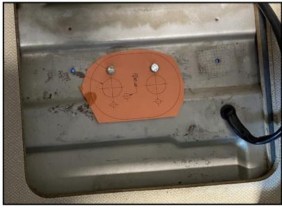
8) Mark the location of the final five holes using a center punch. Drill 1/8" holes in each location, then drill to the final size with the appropriate drilling tools. It helps to use the metal plate in the kit for accuracy. See image below.
