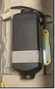
10) Apply hi-temp silicone around the holes on the underside of the vehicle, and secure the heater with four serrated nuts.
