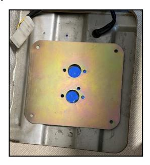
9) Place the steel plate at the bottom of the heater and align the studs and tubes into the holes in the van.
