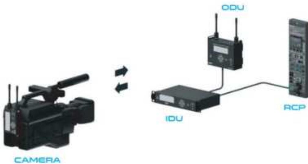
Figure 4:Wireless Camera System configuration
