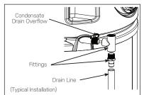
**WATER SUPPLY CONNECTIONS:** Refer to the illustration below for suggested typical installation. The installation of unions or flexible copper connectors is recommended on the HOT and COLD water connections so that the water heater may be easily disconnected for servicing if necessary. The HOT and COLD water connections are clearly marked and are 3/4" NPT on all models.
