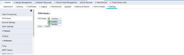
d) Confirm that an automatic restart of all ISE services will take place as ISE initializes the cryptographic library into FIPS 140 mode, by clicking on the **OK** button.
