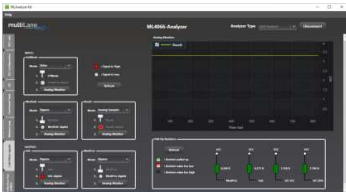
Figure 17: Reading ResetL from the Analog Monitor Window
