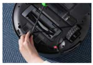
Gently tap and rotate both wheels to check for obstructions. Remove any debris if necessary.
