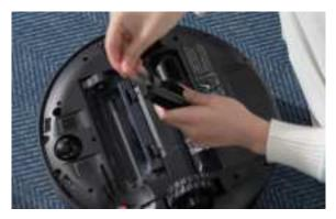
• If the swivel wheel is jammed with dirt or hair, remove it and clean it thoroughly.
