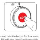
Press and hold the button for 5 seconds, and the LED indicator light Flashing rapidly .
