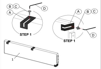
**STEP 2:** Attach brackets (A) facing right side to wing, to the end of the slot, using wrench(D), screw (B), and flat washers (C).
