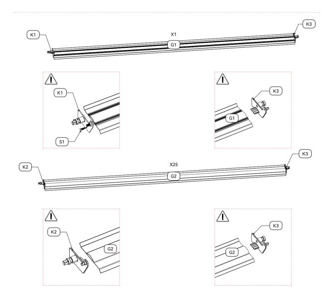
Assemble the master louvre(G1), please note to install one end of it and then connect the other end.
