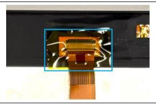
Disconnect LCM FPC connector and remove the LCM FPC.
