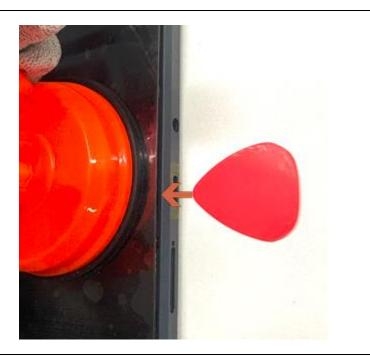
Slide the plastic plectrum along the edge of the screen according to figure's arrow direction.
