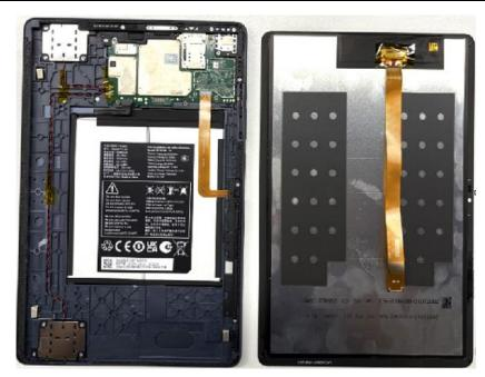
Remove the LCD connector Mylar.
