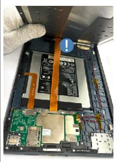
Remove cross-head screws from LCD BTB Fix STEEL.
