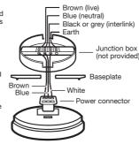
If desired, the alarm can be interconnected with up to 11 other smoke, heat or carbon monoxide alarms from the FireAngel range via the 'I' connector. (See Optional Interconnecting Feature)
