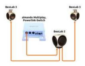
You can also connect a subwoofer. The subwoofer itself has two further Powerlink sockets to which you connect the pair of speakers.
