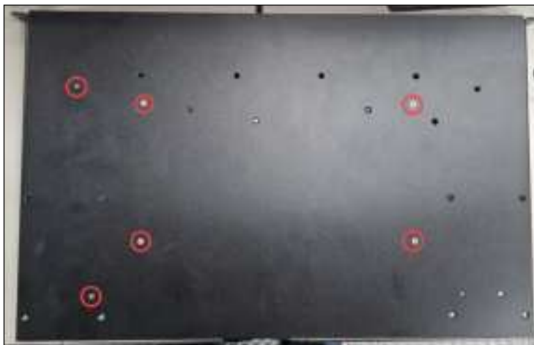
Figure 3: Bottom View of Rack Mounting
