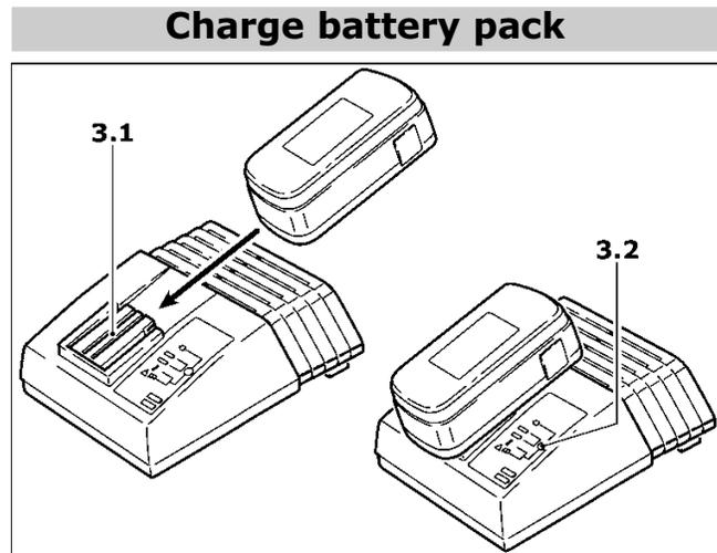
To load the battery pack, push it into the holder (3.1) on the charger up to the stop. Perform this in reverse to remove the battery pack from the charger.
