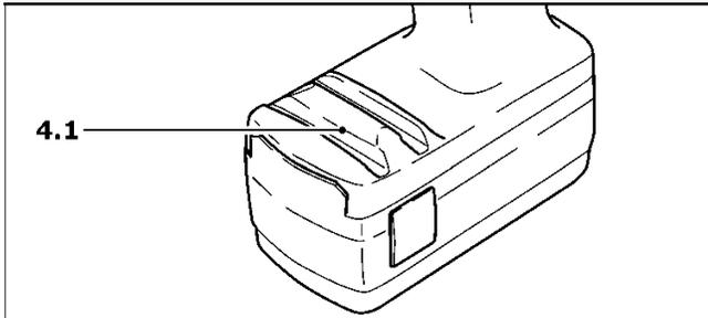
You can insert several bits or bit extensions into the bit magazine (4.1) from the side.
