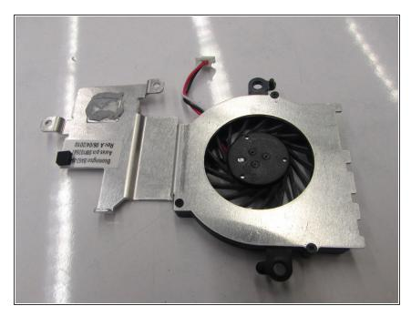
Remove the metal casing with the fan attached from the motherboard.
