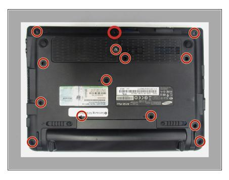
Using the Phillip's 00 screwdriver, unscrew the fourteen 7mm screws until the back panel comes loose.
