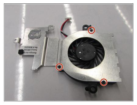
• Use the Phillips #000 screwdriver, to unscrew the three 4mm screws.
