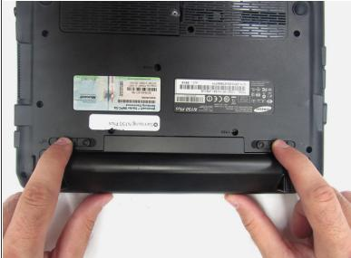
• Slide the left and right switch to the "unlocked" position.
