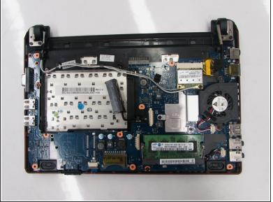
The computer should be open with the motherboard exposed and internal components exposed.
