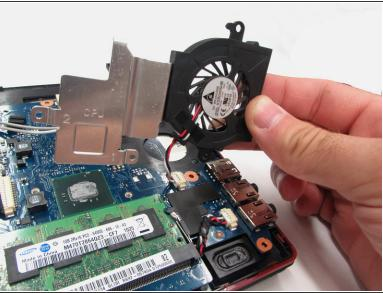
• Use the phillips #00 screwdriver, to unscrew the two 5mm mounting screws labeled 1 & 2 on the right and left hand side of the metal casing labeled CPU.
