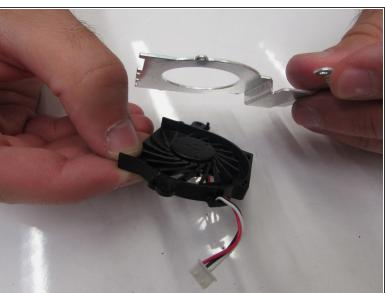
• Remove the fan from the metal CPU housing.
