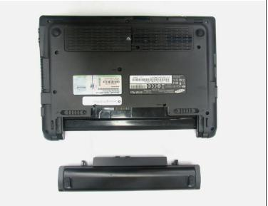
• While holding the left and right hand switches in the "unlocked" position, push the battery away from the computer.
