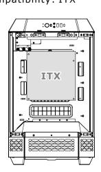
CPU cooler max height: 210mm
