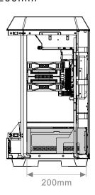
VGA max length: 245 mm (With Power Cover) 360 mm (Without Power Cover)
