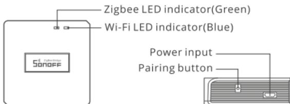
⚠ The device weight is less than 1 kg. The installation height of less than 2 m is recommended.
