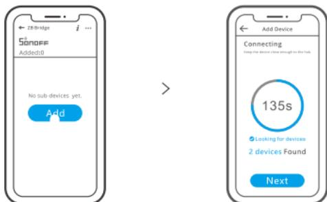
Make the sub-devices enter the pairing mode, tap “Add” icon on the Zigbee Bridge interface, then wait it to find the sub-devices and pair.
