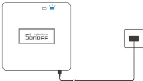
Power the device through Micro USB cable. After powering on, the device will enter the Pairing Mode during the first use. The Wi-Fi LED indicator changes in a cycle of two short and one long flash and release.
