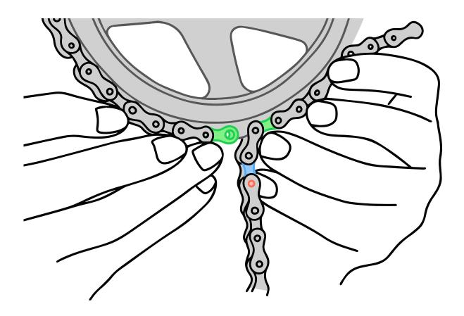
Cut the chain using a chain breaker.
