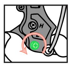
Adjust the **B-tension screw** until there is **5-6mm** of distance between the guide pulley and the tallest teeth of the largest cog.
