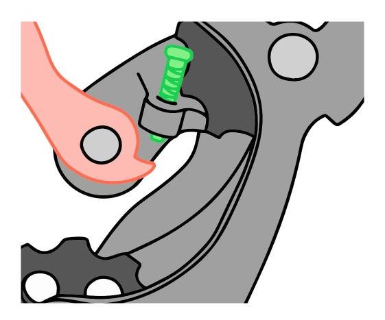
Tighten the rear derailleur fixing bolt to 8 - 10Nm with a 5mm hex bit. Check to make sure that the derailleur can rotate freely.
