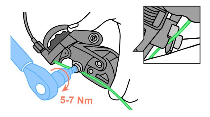
Cut the cable and attach the cable end.
