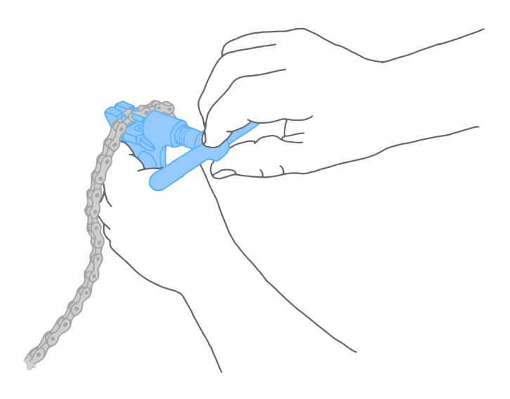
Route the chain over the smallest cog, in front of the guide pulley, behind the derailment prevention plate, and behind the tension pulley. Wrap the chain around the chainring and connect the chain according to the chain manufacturer's instruction manual.
