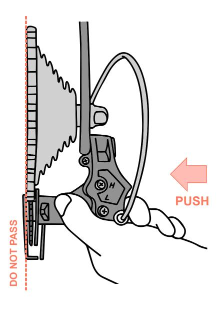
Tighten the **low limit screw** until you can't move the derailleur past the largest cog. Shift down and back up to the largest cog. If it is slow to shift to the largest cog, loosen the low limit screw.
