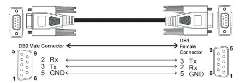
■ Connect a AS-PLC to TP02G via DB9 (MALE) to DB9 (FEMALE) standard cable
