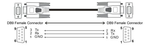
■ Connect a DVP-PLC to TP02G via cable UC-MS010-02A(1M)/UC-MS020-01A(2M)/UC-MS030-01A(3M)
