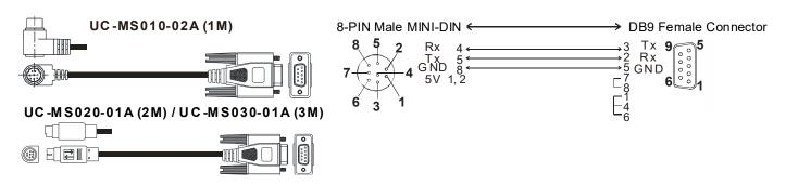
■ Connect a AH-PLC to TP02G via cable UC-MS030-03A(3M)
