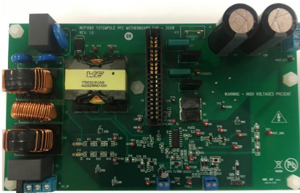
Figure 1. NCP1680 Evaluation Board
