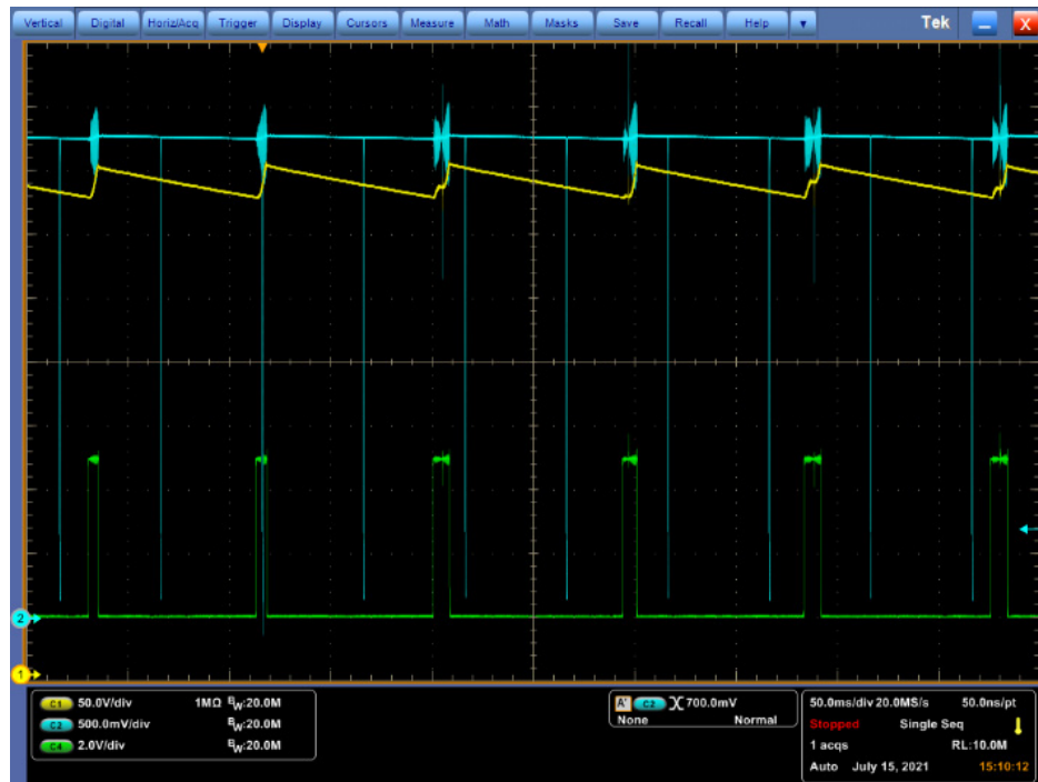
Figure 14. NCP1680 Skip Mode Operation (Ch1 = Bulk Voltage, Ch2 = PFCOK, Ch4 = SKIP)
