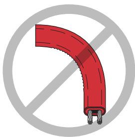
Figure 7: Bending the SC heating cable
