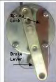
Brake lever released
