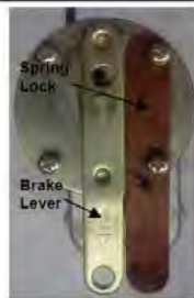
Brake lever engaged
