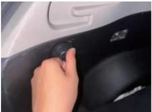
Secure the mounting B to the vehicle. Do not fully tighten to allow adjustability. Repeat this step on the other side of the vehicle.
