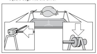
6 Insert the grill tray and the rotisserie spit on the lowest level of the oven. The drive shaft has to engage into the opening on the back of the oven interior.
