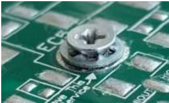
Properly installed and seated screw and washer
