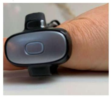
This is how you swap in and out of "mouse mode" with Tap. When your mouse is on the surface you will have a different set of Tap commands. When you are ready to switch back into input mode (entering text, symbols and numbers), simply lift your thumb off the surface and your Tap will automatically swap.
