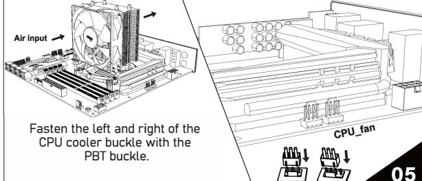
Fasten the left and right of the CPU cooler buckle with the PBT buckle.
