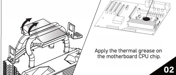
Apply the thermal grease on the motherboard CPU chip.
