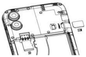
Following the instructions illustrated in above picture, you can insert the Nano SIM card into the SIM compartment with gold contacts facing down, or remove the SIM card by pushing the top of SIM card from opening and pull it out.
