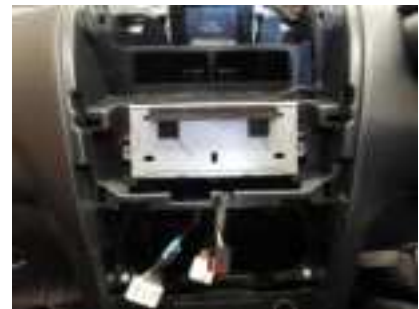
9. Remove 2 screws holding the CD housing in place
