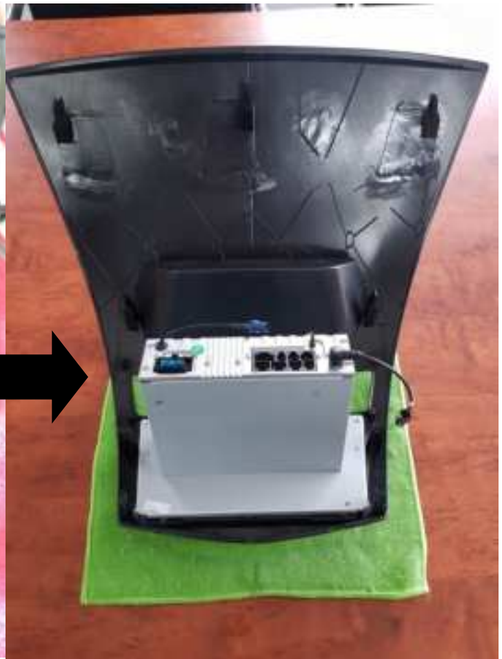
2. Attach clips to new fascia panel
