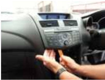
4. Use trim tool to remove fascia panel
