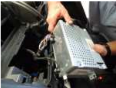
10. Unplug harness and set CD housing aside
