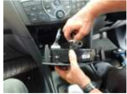
3. Unplug harness and set air con panel aside
