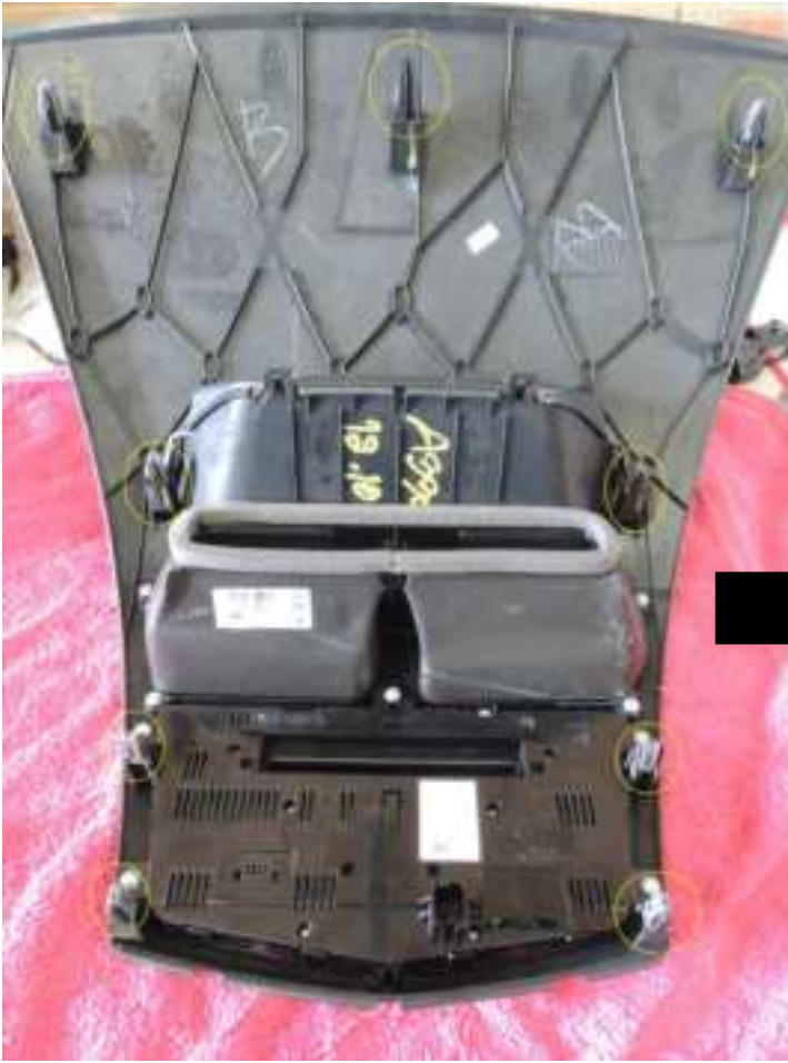
1. Remove clips from original fascia panel...
