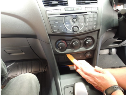
1. Use trim tool to remove air con control panel
