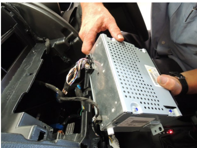
10. Unplug harness and set CD housing aside
