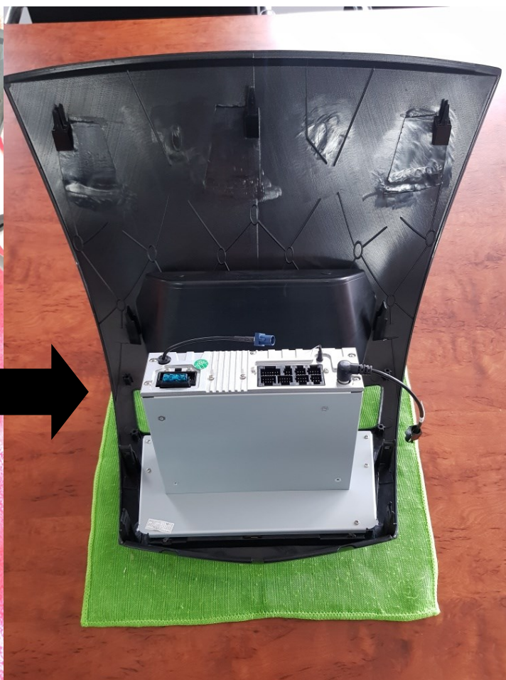
2. Attach clips to new fascia panel
