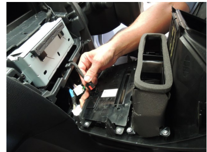
6. Unplug button panel and set aside
