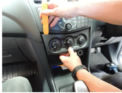
2. Pull Air conditioning panel out.
