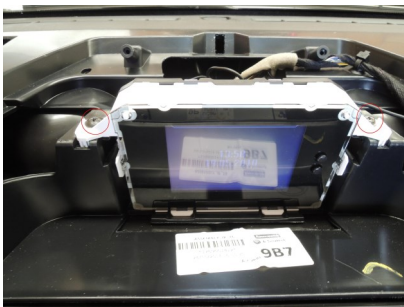
7. Remove 2 screws holding OEM screen in place
