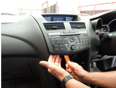
4. Use trim tool to remove fascia panel
