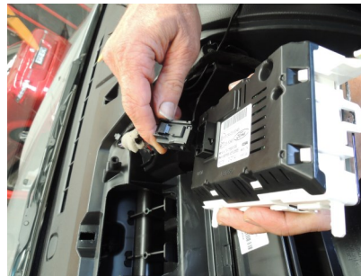
8. Unplug harness and set screen aside
