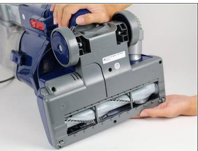
Lay the vacuum down by hand and locate the roller brush underneath the vacuum cleaner.
