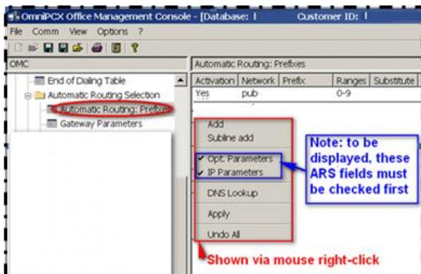
As illustrated in the following picture, first insert a route-line for standard calls (i.e. national/ international numbers): use the Add function to create a new line and then, configure the line parameters as indicated.
