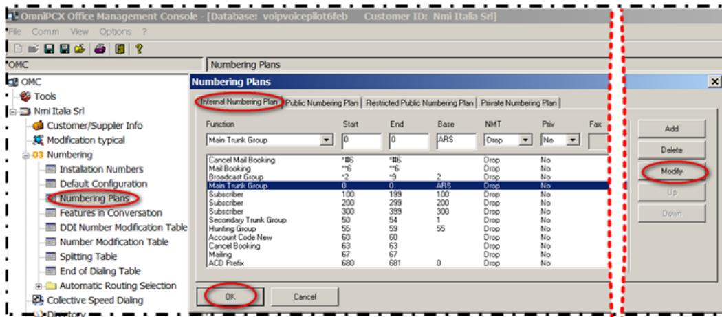
This example defines access to the internal ARS table for user dialing starting with digit 0. The "Drop" attribute indicates that the number dialed must be analyzed in the ARS Prefix table after dropping the initial digit 0.
