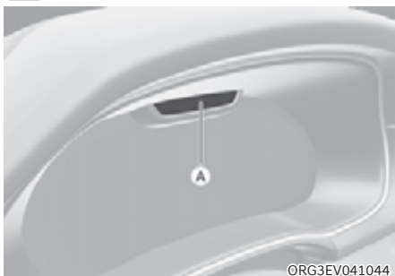
[A] : Interior view camera
