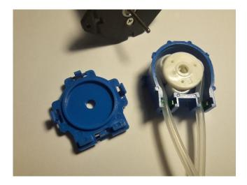
Take out the rollers and the tube. This tube can be replaced by our VMA448.
