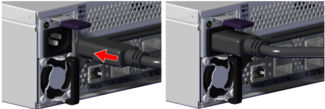
Figure 158: Connect Power Cable
