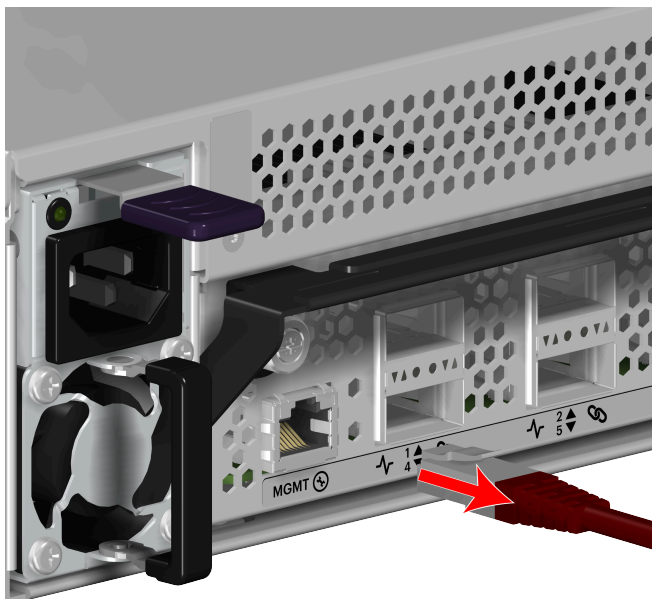
Figure 61: Disconnect Ethernet Cable
