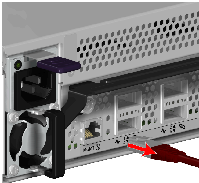
Figure 80: Disconnect Ethernet Cable
