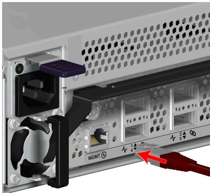
Figure 122: Connect Ethernet Cable
