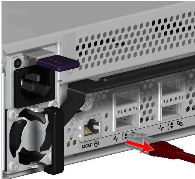
Figure 50: Disconnect Ethernet Cable
