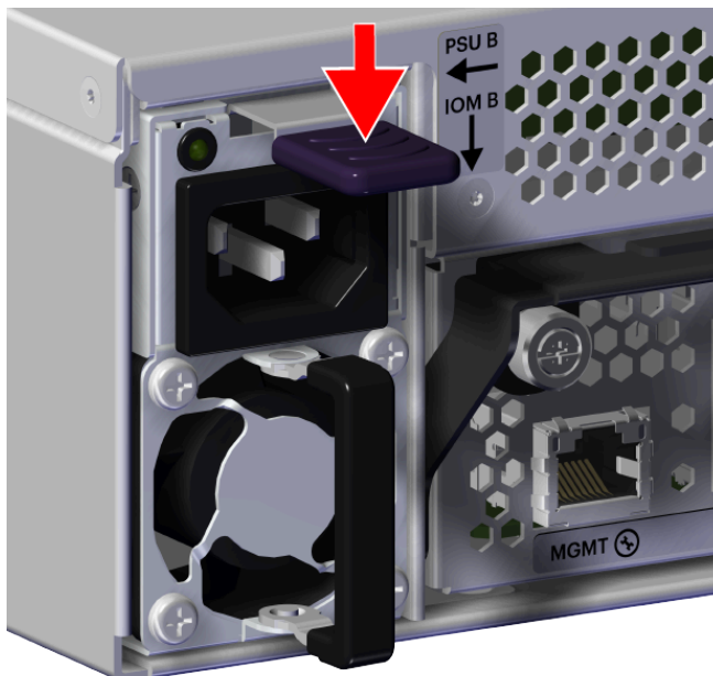
Figure 131: PSU Release Latch Operation
