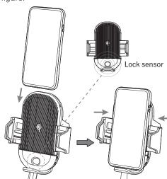
The lock sensor senses the smartphone and the sliding arms close automatically.
