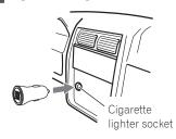
Use the supplied USB charger to perform quick charging. Quick charging may not be possible with a charging port fitted to the vehicle as standard or a commercially available USB charger with an insufficient voltage/current because USB output equivalent to the product input specification is required.
