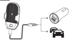
When inserting the USB connector into this product, insert it until you hear a click. When the cable is connected, the power lamp and charging lamp will illuminate. For details on illumination status, see "Product Status Display".
