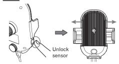
The sliding arms widen automatically. If the product does not operate, start the vehicle's engine and then perform the operation.
