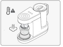
6. A hot shot of water will be dispensed. While the hot shot is dispensing the Power button (N) will be flashing.
