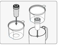
2. Insert filter into the filter hopper and insert filter hopper (C) into water jug.
