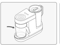
Place an empty container under the water outlet, with at least 1 litre capacity.
