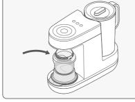
**8.** Remove the lid and place your bottle back on the stand. Press the Power button (N) again to dispense the remaining water.
