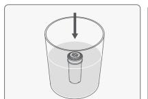
1. Prime your filter by submerging upright it in a bowl of cold tap water. Tap the base of the filter to remove any air bubbles for 5 minutes.
