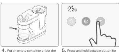
5. Press and hold descale button for 2 seconds. If you need to pause, press the button again. Press and hold the same button for 2 seconds if you need to cancel.
