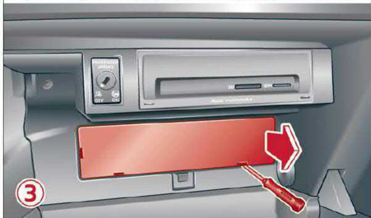
Fig. 170 Left side of the cockpit: storage compartment (left-hand drive) ② or storage compartment (right-hand drive) ③
