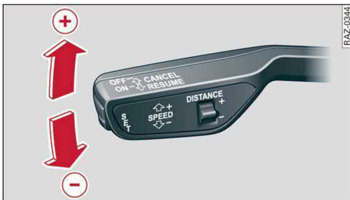
Fig. 97 Operating lever: changing the speed
