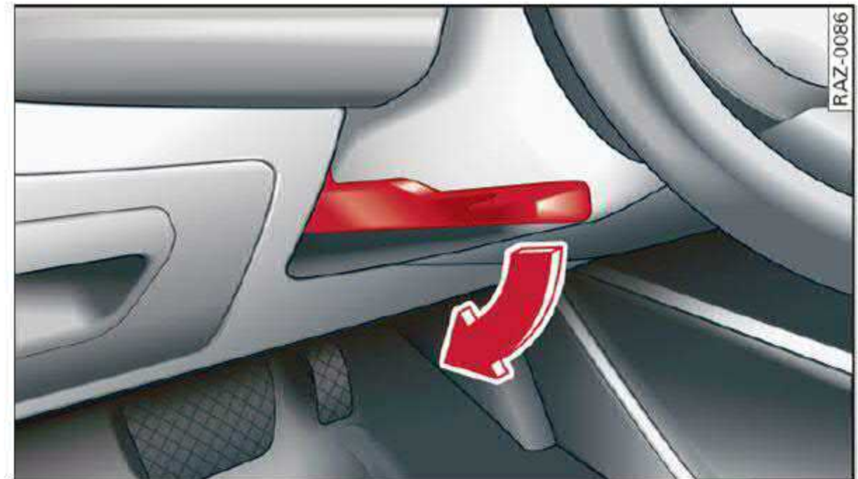
Fig. 53 Steering column: lever for adjusting the steering wheel position
