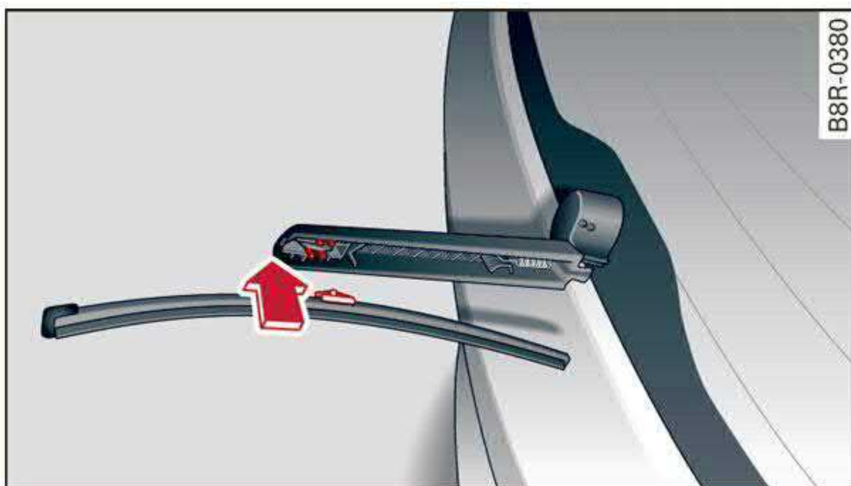
Fig. 46 Rear window wiper: installing the wiper blade
