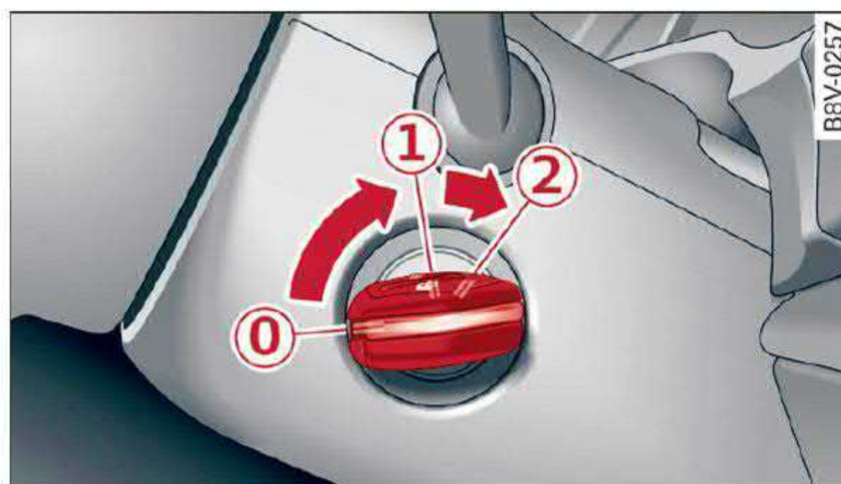
Fig. 79 Steering column: ignition lock
