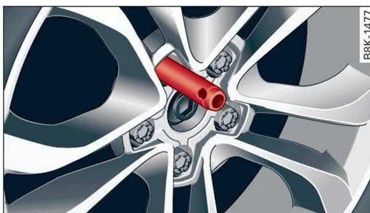
Fig. 163 Wheel: alignment pin in the top hole
