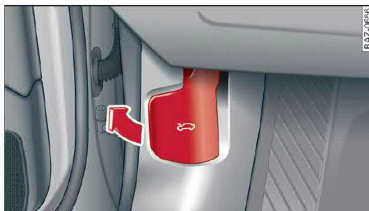
Fig. 143 Footwell: release lever
