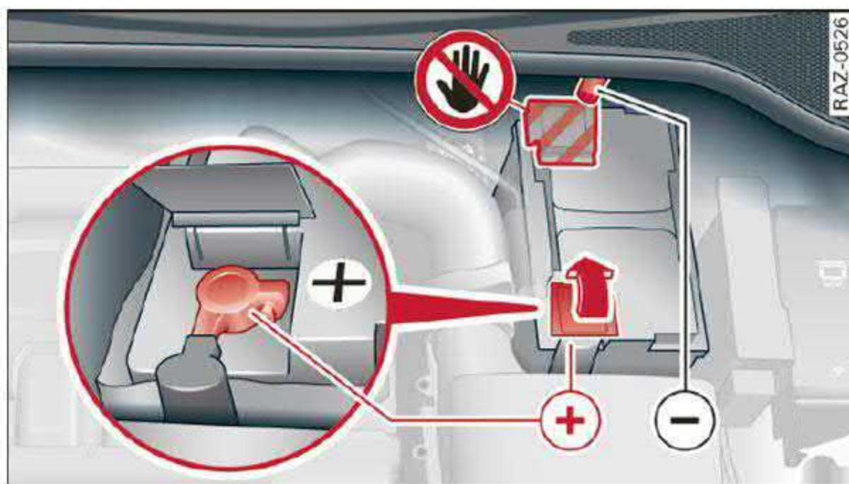
Fig. 150 Engine compartment with battery: connections for charger and jump start cable
