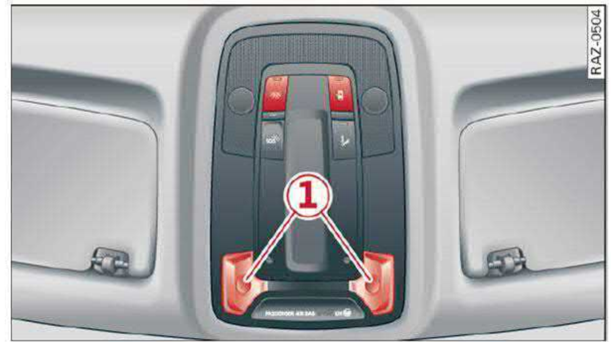
Fig. 39 Headliner: interior lighting
