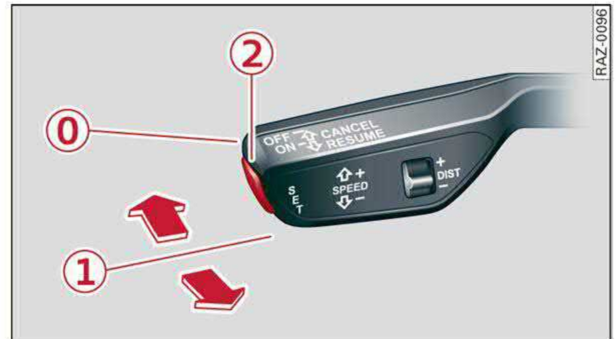
Fig. 100 Lever: overriding the control
