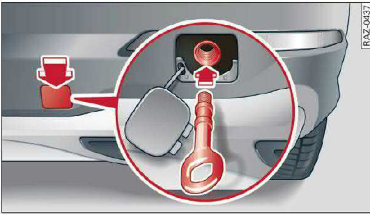
Fig. 168 Rear bumper: installing the towing loop
