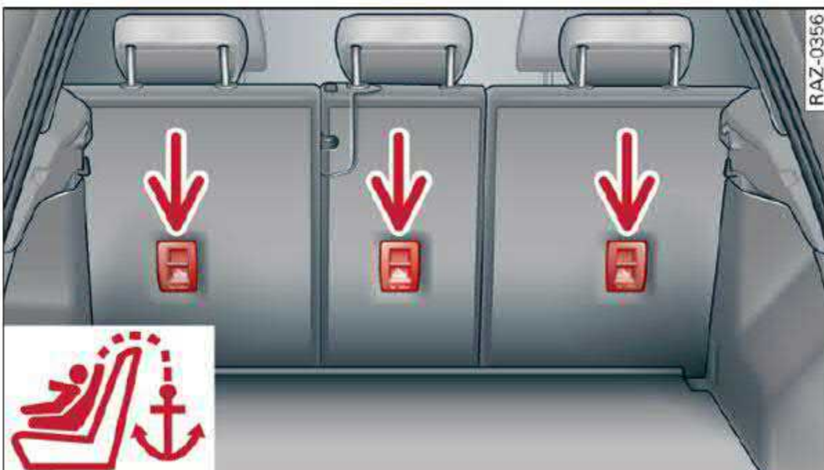
Fig. 65 Rear backrest: top tether anchors to secure a child safety seat with an upper belt
