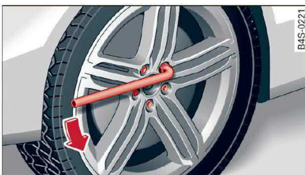
Fig. 159 Wheel: loosening the wheel bolts
