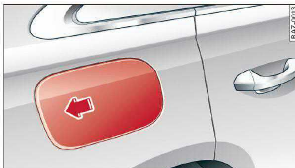
Fig. 140 Right rear side of the vehicle: opening the fuel filler door
