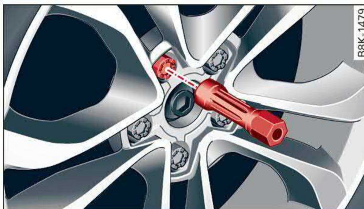
Fig. 162 Wheel: internal hex socket to turn the wheel bolts
