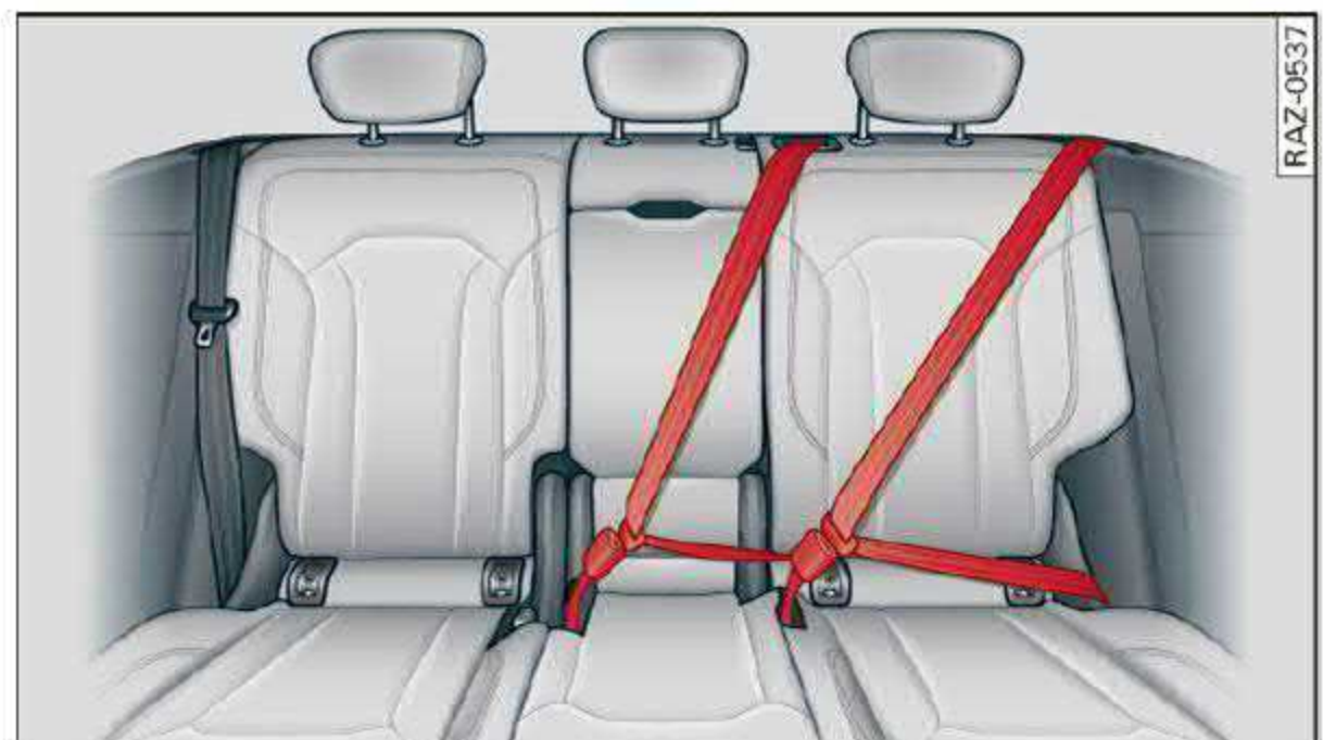
Fig. 67 Rear bench seat: securing unused safety belts
