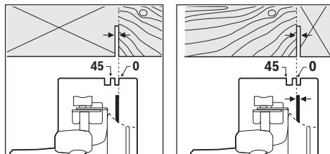
The 0° cut mark (10) indicates the position of the saw blade when making a right-angled cut. The 45° cut mark (9) indicates the position of the saw blade when making a 45° cut.
